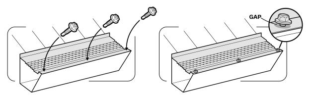
For proper performance, install screws straight and do not overtighten. Once installed, there should be a small gap below the round washer head of the screw for the clip to attach.
